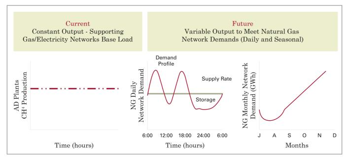
Figure 15. Current and future operation of AD plants to match biomethane production with the gas grid demand.
