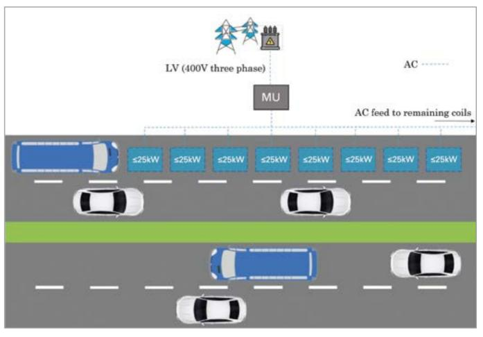
Figure 15. Electron system architecture for a single management unit (MU) network interface, direct to dedicated substation.
