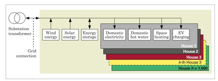
Figure 2. Energy model architecture (Sprake, 2023).
