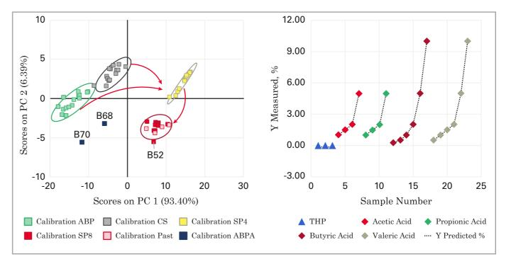
Figure 8. A. Characteristics of a plug flow reactor's feedstocks (animal by-products (ABP) – food wastes), cattle slurry (CS), intermediates (fermentates SP4), digestate (SP8), and post pasteurisation (past). B. Speciated VFAs measured and predicted at various concentrations.
