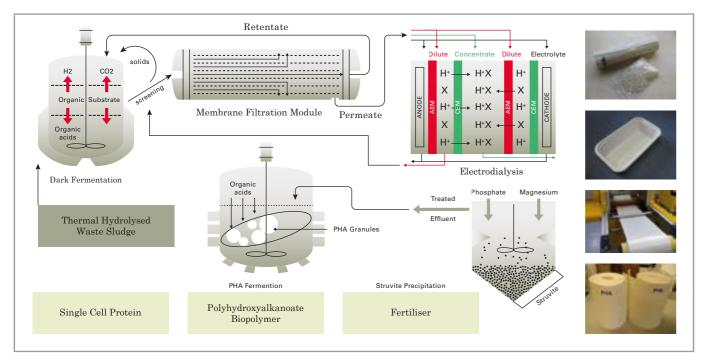
Above: Figure 23. Bioprocess development for valorisation of sewage sludge into SCP, PHA and a fertiliser (left) (adapted from Tao et al., 2014). Processing PHA into products (e.g. pellets, films, trays) (right) (source: Biocomposite Centre).
